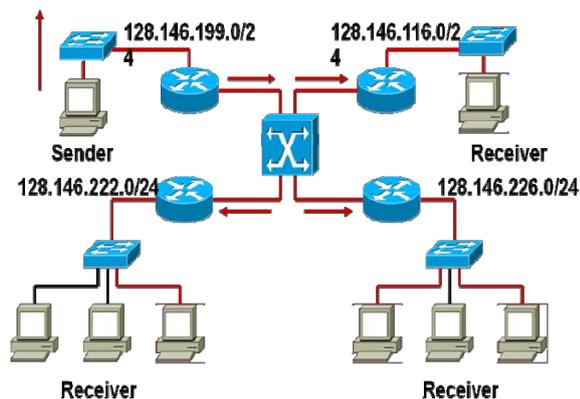
Fig 2: Multicast Routing
